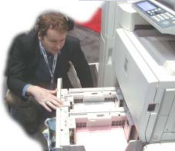
BERTL analyst inspecting Sharp AR-M620's 2,000-sheet tandem drawer paper supply
